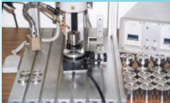
Laser welding of diaphragms.
